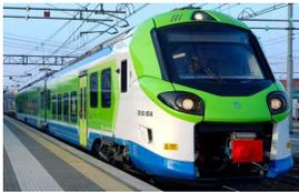
Target of the project is to convert the actual line today served by diesel trains in a completely «green line» operated by ALSTOM hydrogen trains
